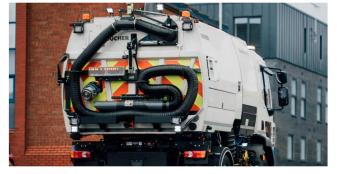
A long seven metre reach Littasnatch option with air operated gate designed for the collection of lightweight debris in hard to reach places.
