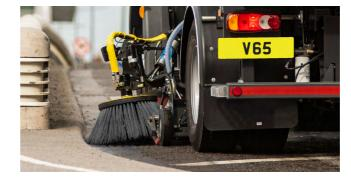
Rotatilt option adjusts the angle of the channel brush from the cab to clean crevasses and cambered roads.
