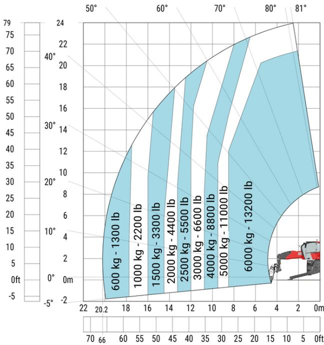
Machine on lowered stabilisers with winch 7200 kg (metric)
