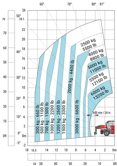
Machine on lowered stabilisers with forks Metric
