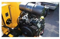
**25 HP (18.6 KW) EFI ENGINE.** Performs well during cold-weather starts, has reduced occurrence of engine flooding and provides improved fuel economy over comparable carbureted gas engines.
