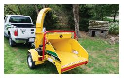
**LARGE INFEED OPENING.** The 6" x 8" (15.2 cm x 20.3 cm) infeed opening makes feeding irregular material easier and decreases the amount of saw cuts needed prior to feeding the chipper.
