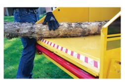
**ELECTRONICALLY SWITCHED BOTTOM FEED STOP BAR.** Strategically located to make it possible for the operator's leg to strike the bar and shut off the feed roller, either intentionally or automatically in an emergency situation, increasing operator safety while feeding material.
