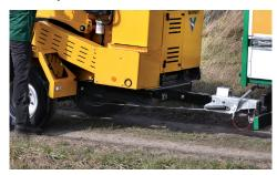
**EUROPEAN UNDERCARRIAGE WITH SURGEBRAKE.** The full type approved European undercarriage comes with a Knott axle and surge brake. The heavy-duty undercarriage provides good towing performance on-road.
