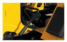
**CLUTCHLESS PTO SYSTEM.** A clutchless PTO system reduces premature wear to the belt drive system by preventing high-speed engagement of the cutter drum. The throttle is integrated with the belt drive to help ensure the PTO can be engaged only while the engine is at low speed.
