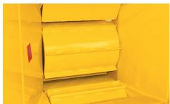
**DUAL OFFSET FEED ROLLERS.** Dual horizontal offset feed rollers improve performance by grabbing and feeding material to the drum. The offset helps the upper feed roller climb over big logs or material with multiple (forked) branches.
