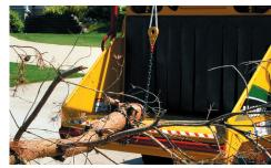
**EASILY LIFTS HEAVY MATERIAL.** An optional winch allows operators to move large logs effortlessly. The winch line can handle up to 900 kg and can be used to lift logs onto the feed table.
