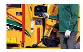
**CONTROL PANEL AND HYDRAULIC CRUSH** LEVER. Hydraulic crush lever provides an aggressive grip when dealing with difficult material. Our exclusive SmartFeed system automatically monitors engine speed and stops or reverses the feed rollers if needed, reducing strain on the engine.
