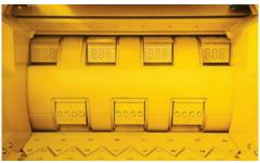
CHIP PRODUCTION. The optional chip drum produces a consistently chipped end product, rather than traditional shredded material, for uses such as biofuel.
