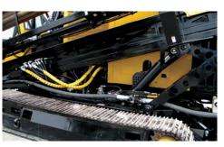
**INCREASE YOUR RANGE.** Unique four-bar linkage rack and additional pads allow operators to set up entry angles of 11 - 24° — increasing range attainable with tracks fully on ground.
