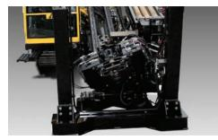
**OPEN-TOP VISE.** An angled, open-top vise allows for the passage of larger tooling. Because of the large opening, operators can also use it to break out tooling.
